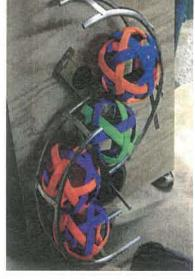
Inventor® was used to plan an all aluminum version. Using a conduit bender, 5/8" diameter aluminum tubing was bent into three "C's". A wooden jig was built to hold them in place for welding.
